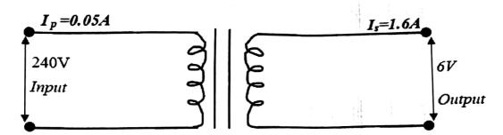
(i) If the number of turns in primary coil is 240. Determine the number of turns in the secondary. (2mks)
