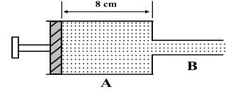
If the piston travels the length, 8 cm in 2 s, determine the velocity of the liquid in section B.
