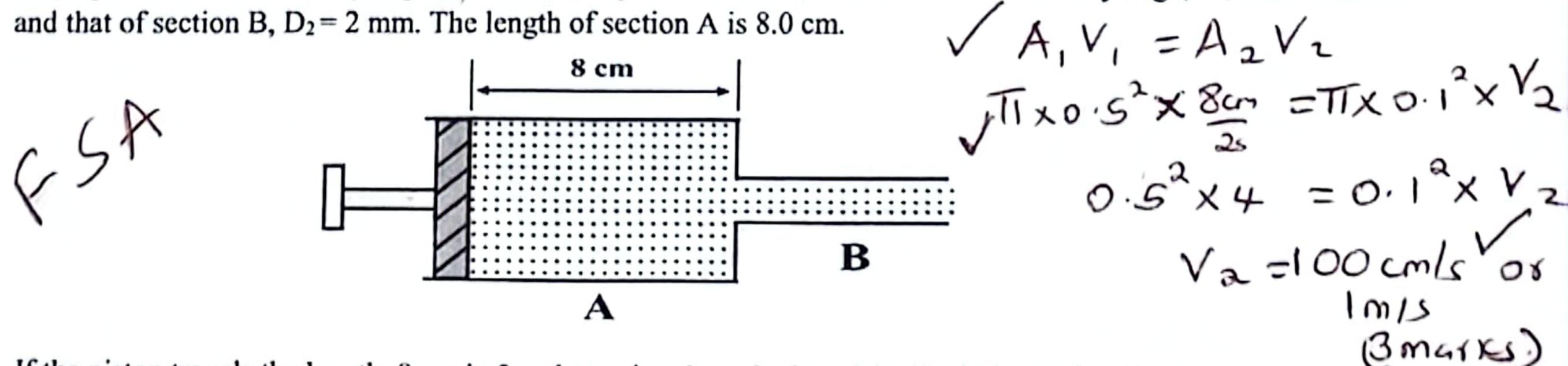
If the piston travels the length, 8 cm in 2 s, determine the velocity of the liquid in section B.
