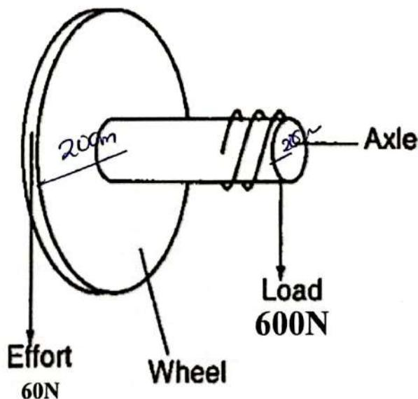
If the radius of the wheel is **20cm** and that of axle is **2cm**, determine the machine's:
